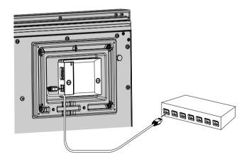
The AC cord must be disconnected from AC power outlet when connecting the cable. It may damage the product.
